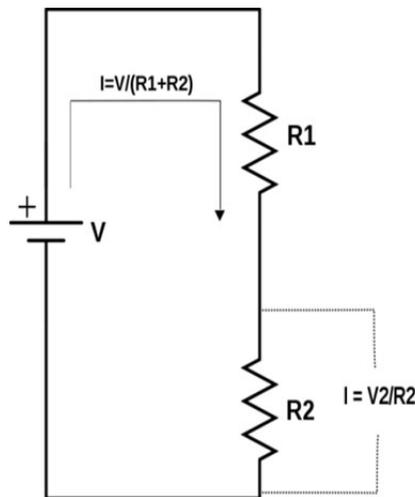
$$V_2 = R_2 / (R_1 + R_2) \cdot V$$
