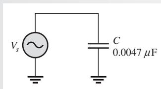
**Solución**  $X_C = \frac{1}{2\pi fC} = \frac{1}{2\pi(1 \times 10^3 \text{ Hz})(0.0047 \times 10^{-6} \text{ F})} = 33.9 \text{ k}\Omega$
